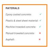
Air casters need to build up pressure between the air chamber and the floor. Therefore, the surface needs to be non-porous and have a smooth finish. Most facilities have a machine trowelled concrete floor, that will work perfectly. The table on the left shows roughly what surfaces will and will not work. A rougher, more porous surface will result in more air consumption.
