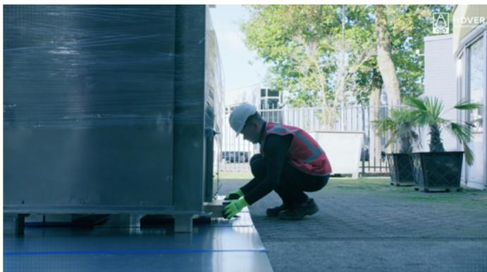
Place the air control unit in the most logical position to perform the movement. Mostly the unit is placed in front of the object in the direction of the movement. Or on one of the sides if that is more practical.
