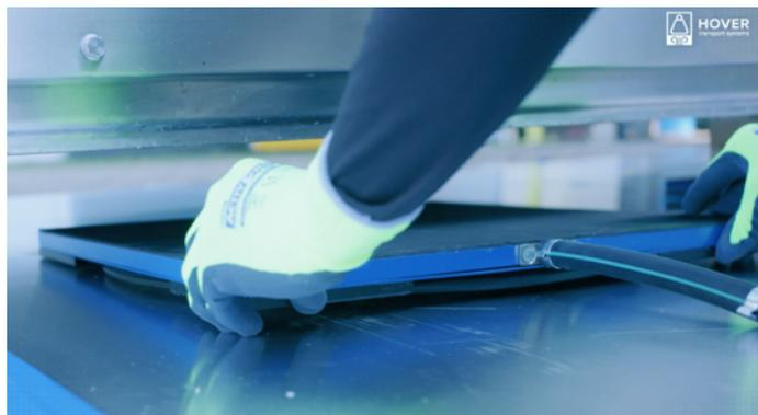
Next fill out the gap out (if there is one) with wooden or plastic beams or plates. Fill the gaps out until there is ideally less than 0,5cm (0,2") of open space between the air caster assembly (with the air casters deflated, so with the black landing pads on the floor) and the object.
