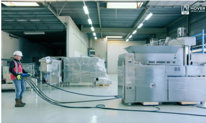
Move the load safely to its destination and frequently check the state of the air caster assemblies and the load itself.
