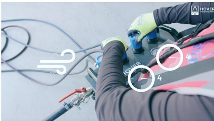
When all air casters have lifted the load from the landing pads, finetune the flow for each air caster individually until they all hover above the floor.
