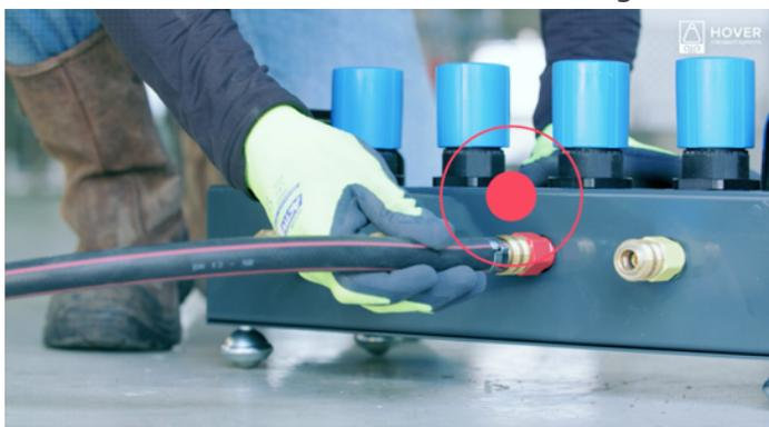
Before you connect the air supply hose to your air supply system, make sure that the air flow is completely closed!
