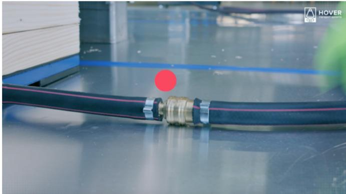
Connect the air interconnect hoses to the air control unit and make sure that the colour code is matching.
